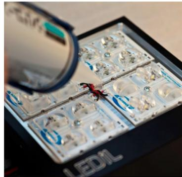
Only apply potting compound outside the optical areas. STRADA lenses for example are designed with barrier walls to keep the compound out of the lenses.
