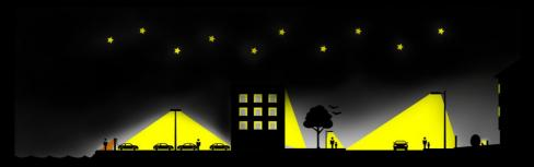
Well designed luminaires and the right optics can reduce light pollution and skyglow.
