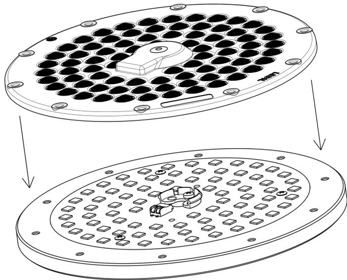
4. Fix the lens with M4 screws
