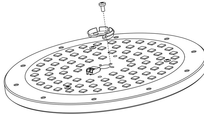
3. Push lens down to clip and rotate position pins to match corresponding holes in PCB
