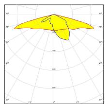
Dimensions: 49.5 mm x 49.5 mm Height: 5.00 mm IESNA Type III (medium) beam for
