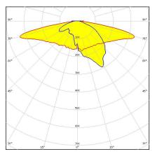
Dimensions: 49.5 mm x 49.5 mm Height: 5.70 mm IESNA Type III (medium) beam for
