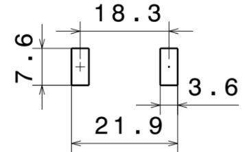
Clip reference distance after soldering
