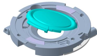
1. slid in one side of the RZ lens "legs" to HEKLA SOCKET locking features
