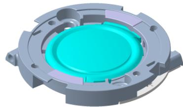
2. Bend the RZ lens and slid in other side of the RZ lens "legs" to HEKLA SOCKET locking features
