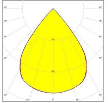
Dimensions: 1140.0 mm x 40.0 mm Height: 20.20 mm ~80° wide beam. Variant with diffused 7X1 lenses.
