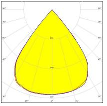
Dimensions: 1140.0 mm x 40.0 mm Height: 20.20 mm ~80° wide beam. Variant with 4X1 lenses.
