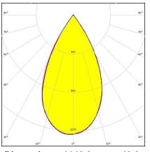
Dimensions: 1140.0 mm x 40.0 mm Height: 20.20 mm ~50° wide beam. Variant with 4X1 lenses.
