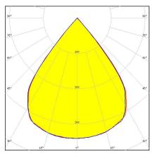
Dimensions: 1140.0 mm x 40.0 mm Height: 20.20 mm ~80° wide beam. Variant with 7X1 lenses.
