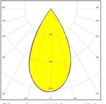
Dimensions: 1140.0 mm x 40.0 mm Height: 20.20 mm ~50° wide beam. Variant with diffused 7X1 lenses.
