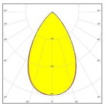
Dimensions: 1140.0 mm x 40.0 mm Height: 20.20 mm ~50° wide beam with tighter cutoff. Variant with diffused 7X1 lenses.
