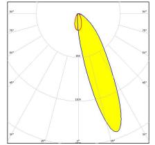
Dimensions: 21.5 mm x 21.5 mm Height: 16.10 mm Asymmetric beam for wall-washing. Assembly with holder and installation tape.
