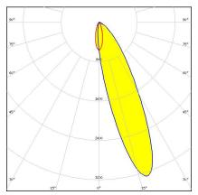
**Dimensions: 21.5 mm x 21.5 mm Height: 16.10 mm** Asymmetric spot beam with ~17° tilt for billboards. Assembly with holder and installation tape.
