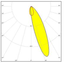
Dimensions: 21.5 mm x 21.5 mm Height: 16.10 mm Asymmetric beam for billboards. Assembly with holder and installation tape.
