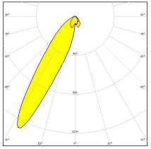
Dimensions: 49.9 mm x 49.9 mm Height: 13.60 mm Asymmetric beam for wall washing
