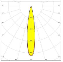
Dimensions: 49.9 mm x 49.9 mm Height: 10.80 mm ~18° spot beam
