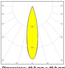
Dimensions: 49.9 mm x 49.9 mm Height: 10.91 mm ~24° medium beam
