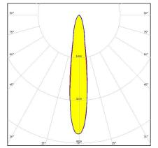
Dimensions: 49.9 mm x 49.9 mm Height: 10.80 mm ~15° spot beam with soft cutoff
