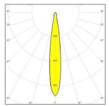
Dimensions: 49.9 mm x 49.9 mm Height: 11.00 mm ~15° spot beam with tight cutoff
